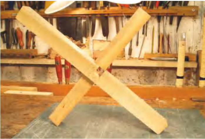
▲ Pic.9 Pieces 1 and 2 now interlocking BUT only halfway through
